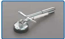
Light, ultra-compact magnetic lifter ideal for quick and multiple lifting of medium/heavy weight covers. With a weight of just 2,5 Kg has an incredible lifting force thanks to the latest neodymium type magnets. Opens and folds with one hand, attaches very strongly to the metal lids and can be easily detached with a lateral stroke. The handle foldability makes it really tiny for easy handling and transportation, can be stored anywhere even under vehicles seats.
