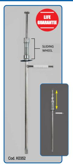
Practical and versatile tool designed to ease the removal of the cover from the manholes frame that are stuck by rust, ice, stones, asphalt incrustations and inactivity. The wedge penetration effect of the tip, between the frame and the cover, creates a strong lateral pushing force that splits easily the incrustations formed by sediments that block the opening, just a couple blows and the separation/detachment is done, fast, powerful and safe.
