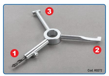
T3 POLY TOOL is a clever multi purpose tool designed to make the typical operations needed before to open the covers of manholes, the three extremities have different configurations that allows to drill and scrap, to grab, to open the latches that lock some covers and allow to lift and remove manhole covers Tool is delivered in a robust "cordura" pouch, studied to ease the operations T3 POLY TOOL is an effective and sometimes irreplaceable tool in operation of manoeuvers of manhole covers.
