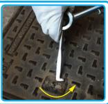
Use the "T" extremity as insertion hooking key in the slots, grabbing then tool as handle to lift by hands or using a chocking belt to lift standing up.
