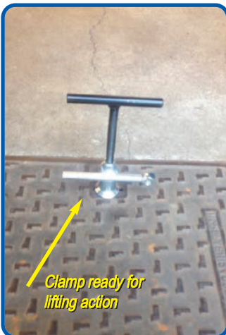
Engagement of the lever in the clamp
