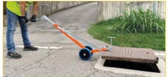
**Use 3:** mechanical opening with locking clamps.
