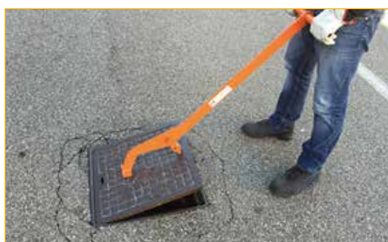
In the opening operation, the length of the lever limits the operator effort.
