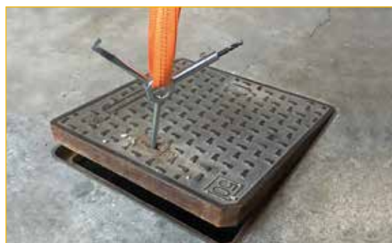
Configuration 4: use in synergy with a choke belt for lifting operations
