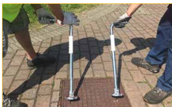
Useful for dividing the effort between two operators in complete safety.
