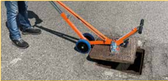
Use 1: opening with magnetic CL9 - CL10 - CL11.
