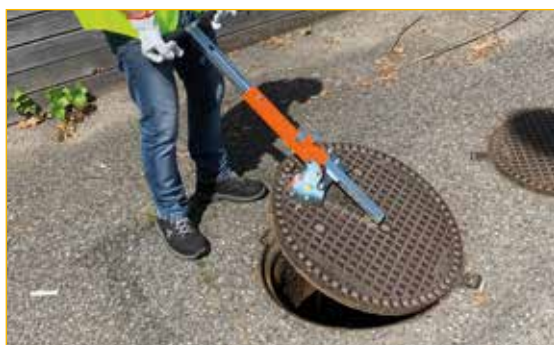
Use 3: Opening with horizontally extended handle bar.
