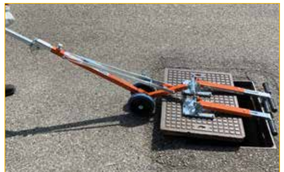
Use 3: opening with two plates in parallel position.
